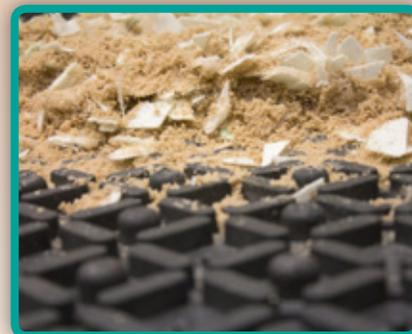
leave a leeway on each side to allow the mat to expand. The mat can expand up to one inch if exposed to the sun, depending on intensity of the sun. Once the footing is spread on the mats, temperature will stay constant underneath the footing. Mat will be more flexible with temperatures above 55 degree and stiffer below this point, but still flexible enough not to crack.
