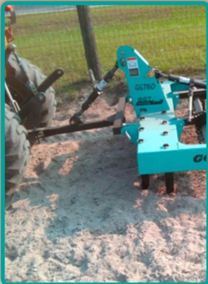
**1 Teeth:** The teeth are designed to break up the ground, intermixing and loosening the footing.
